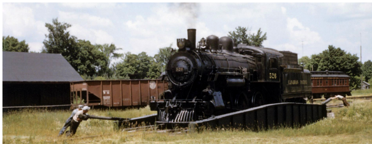
Colour digital photograph of two men turning a train engine on a turntable. CP 526 turning M747 at Elora 28 June 1955. Ph59084 photo courtesy of Wellington County Museum and Archives. Photographer: Robert J. Sandusky
